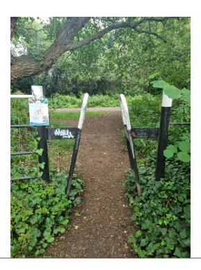
Current A Frame width (Top Width - 36cm Bottom Width -100cm) is not compliant with Equality Act 2010 and restricts some legitimate users in wheelchairs, mobility scooters and adapted cycles.
