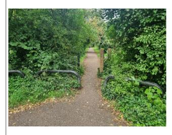
The current width between metal barriers (89cm) is not compliant with Equality Act 2010 and restricts some legitimate users in wheelchairs, mobility scooters and adapted cycles.
